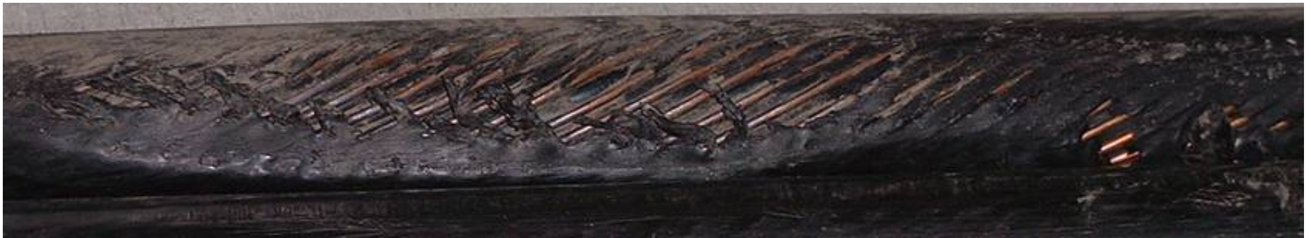
Example: jacket and outer semicon layer stripped during installation
